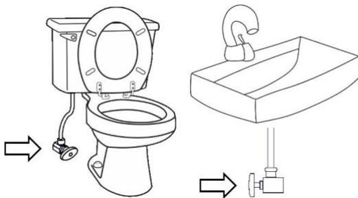
The Aqua-Scope monitors the water pressure and noise by connecting the Aqua-Scope water microphone to the water pipe system. Ideal connection points are edge valves located below sinks or beside toilets. It is recommended to find a place as low in the home as possible (ideally basement or first floor) **but it will work on every place in the home** that meet the following two further requirements:
